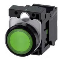
Illuminated pushbutton, 22 mm, round, plastic, green, pushbutton, flat, momentary contact type, with holder, 1 NO, LED module with integrated LED 24 V AC/DC, Spring-type terminal
