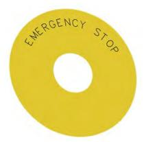
Backing plate round, for EMERGENCY STOP mushroom pushbutton, yellow, self-adhesive, Outer diameter 75 mm, inside diameter 23 mm, with inscription: EMERGENCY STOP
