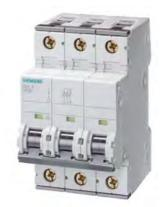
Miniature circuit breaker 400 V 10kA, 3-pole, C, 50 A, D=70 mm
