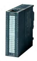
SIPLUS S7-300 SM 322-20-pole -25...+70 °C With conformal coating based on 6ES7322-1BH01-0AA0 . Digital output Isolated 16 DQ, 24 V DC, 0.5 A, total current 4 A/group (8 A/module)
