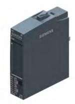
SIMATIC ET 200SP, Digital output module, DQ 16x 24V DC/0,5A Standard, Source output (PNP,P-switching) Packing unit: 1 piece, fits to BU-type A0, Colour Code CC00, substitute value output, module diagnostics for: short-circuit to L+ and ground, wire break, supply voltage
