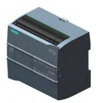
SIMATIC S7-1200, CPU 1214C, compact CPU, DC/DC/relay, onboard I/O: 14 DI 24 V DC; 10 DO relay 2 A; 2 AI 0-10 V DC, Power supply: DC 20.4-28.8V DC, Program/data memory 100 KB
