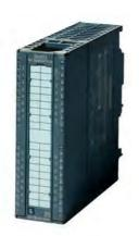
SIMATIC S7-300, Digital output SM 322, isolated, 8 DO (relay), 1x 40-pole, 24 V DC, 5 A or 230 V AC, 5 A, connectors with spring-loaded terminal can be used as of 6ES7392-1BM01-0AA0
