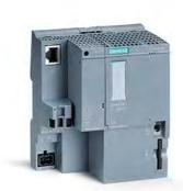
SIMATIC DP, CPU 1510SP-1 PN for ET 200SP, Central processing unit with Work memory 100 KB for program and 750 KB for data, 1st interface: PROFINET IRT with 3-port switch, 72 ns bit performance, SIMATIC Memory Card required, BusAdapter required for Port 1 and 2
