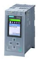
\*\*\* Spare part \*\*\* SIMATIC S7-1500, CPU 1515-2 PN, central processing unit with work memory 500 KB for program and 3 MB for data, 1st interface: PROFINET IRT with 2-port switch, 2nd interface: PROFINET RT, 30 ns bit performance, SIMATIC Memory Card required
