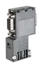
PROFIBUS bus connector, RS 485, screw, with programming port, 90° SIMATIC DP, Connection plug for PROFIBUS up to 12 Mbit/s 90° cable outlet, 15.8x 64x 35.6 mm (WxHxD), terminating resistor with isolating function, With PG receptacle
