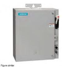
Pump control panel, Size 2, Three phase full voltage, Solid-state overload relay, OLR amp range 13-52A, 110-120/220-240VAC 60Hz coil, Standard type contactor, 50A circuit breaker, HOA Sel Sw. <(>&<)> Start P.B., Enclosure NEMA type 3/3R, Weather proof outdoor use
