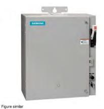
Pump control panel, Size 2, Three phase full voltage, Solid-state overload relay, OLR amp range 13-52A, 220-240/440-480VAC 60Hz coil, Standard type contactor, 50A circuit breaker, HOA Sel Sw. <(>&<)> Start P.B., Enclosure NEMA type 3/3R, Weather proof outdoor use
