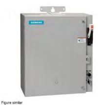
Pump control panel, Size 3, Three phase full voltage, Solid-state overload relay, OLR amp range 25-100A, 110-120/220-240VAC 60Hz coil, Standard type contactor, 100A circuit breaker, HOA Sel Sw. <(>&<)> Start P.B., Enclosure NEMA type 3/3R, Weather proof outdoor use
