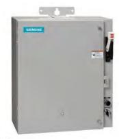
Pump control panel, Size 3, Three phase full voltage, Solid-state overload relay, OLR amp range 25-100A, 220-240/440-480VAC 60Hz coil, Standard type contactor, 100A circuit breaker, HOA Sel Sw. <(>&<)> Start P.B., Enclosure NEMA type 3/3R, Weather proof outdoor use
