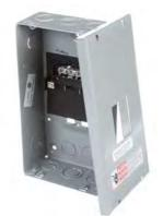
Siemens Energy Management Residential Specialty Load Centers: Small Circuit (2-10). Sub Brand: Load Centers Type: 1: Application: Residential: Voltage Rating: 120/240V Amperage Rating: 60A Phase: 1PH Load Regulation: 60A Wiring Configuration: 3w Bus Rating: 60A Interrupt Rating: 100000AIC. EQ LC 2S 4C ML 60A N1-S
