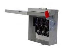
Siemens Low Voltage Circuit Protection General Duty Safety Switches. Type: ENCLOSED, SAFETY SWITCH Std: UL V. Rating: 240V A. Rating: 60A Wattage: 4W No. Of Poles: 3P F. Rating: 60Hz Action: SINGLE THROW Material: STEEL Enclosure: TYPE 1. 2-3 point mounting holes. O. Cycles: 10000 O. Temperature: (-20F-120F) AMBIENT TEMPERATURE Environmental Conditions: INDOOR
