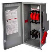
Siemens Low Voltage Circuit Protection Heavy Duty Safety Switches. Type: ENCLOSED, SAFETY SWITCH Std: UL V. Rating: 600V A. Rating: 30 A Wattage: 3W No. Of Poles: 3P F. Rating: 60Hz Action: SINGLE THROW Material: STEEL Enclosure: TYPE 1. 2-3 point mounting holes. O. Cycles: 10000 O. Temperature: (-20F-120F) AMBIENT TEMPERATURE Environmental Conditions: INDOOR
