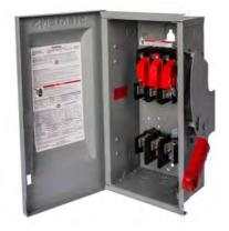
Siemens Low Voltage Circuit Protection Heavy Duty Safety Switches. Type: ENCLOSED, SAFETY SWITCH Std: UL V. Rating: 600V A. Rating: 30 A Wattage: 4W No. Of Poles: 3P F. Rating: 60Hz Action: SINGLE THROW Material: STEEL Enclosure: TYPE 1. 2-3 point mounting holes. O. Cycles: 10000 O. Temperature: (-20F-120F) AMBIENT TEMPERATURE Environmental Conditions: INDOOR
