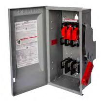
Siemens Low Voltage Circuit Protection Heavy Duty Safety Switches. Type: ENCLOSED, SAFETY SWITCH Std: UL V. Rating: 600V A. Rating: 200A Wattage: 3W No. Of Poles: 3P F. Rating: 60Hz Action: SINGLE THROW Material: STEEL Enclosure: TYPE 1. 2-3 point mounting holes. O. Cycles: 8000 O. Temperature: (-20F-120F) AMBIENT TEMPERATURE Environmental Conditions: INDOOR
