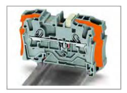
**Step-down jumper (2006-499)** commons 6 /4 mm² (10/12 AWG) terminal blocks (2006 /2004 Series) with 4/2.5/1.5 mm² (12/14/16 AWG) terminal blocks (2004/2002/2001 Series).
