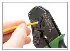
Squeeze handles until ratchet mechanism is released.
