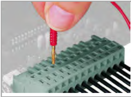
Testing perpendicular to conductor entry via 2 or 2.3 mm Ø test plug – female connector with CAGE CLAMP®.
