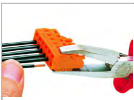
Inserting a conductor via operating tool.
