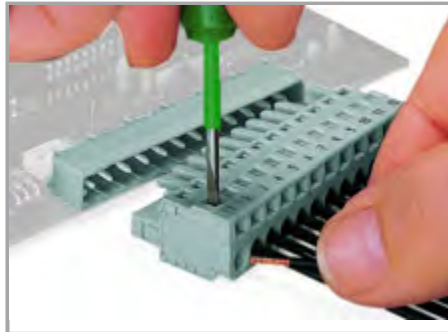
Inserting a conductor via 3.5 mm screwdriver – CAGE CLAMP® actuation perpendicular to conductor entry.
