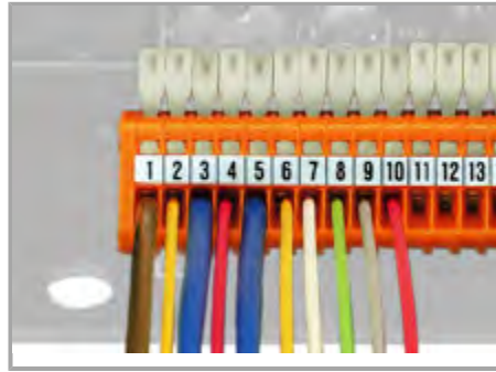
Nominal cross-section: 0.5 mm 2 (20 AWG);
