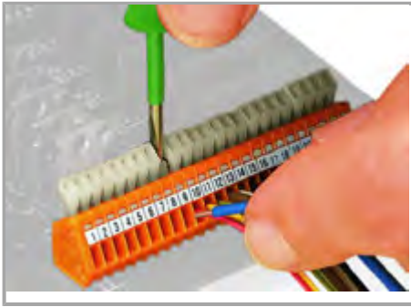
Inserting/removing a conductor.
