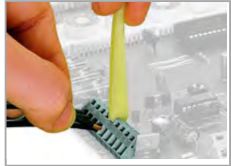
Inserting a conductor via operating tool.
