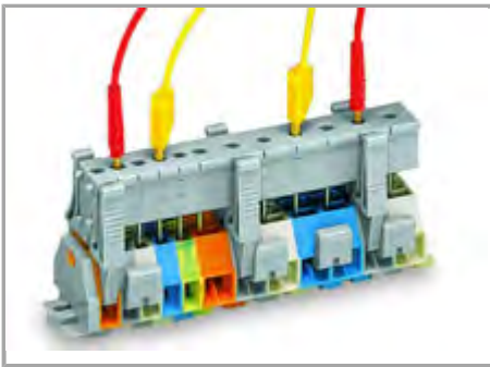
Testing via test plug modules snapped onto a terminal strip – wired or unwired. As touch contact is made with the CAGE CLAMP® (spring steel) unit, this testing type is limited to maximum 0.5 A.
