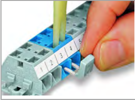
Commoning with comb-style jumper bar.
