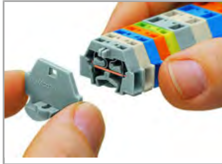
Mounting an end plate.
