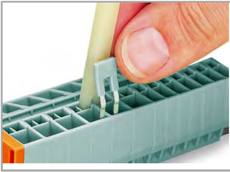
Commoning with comb-style jumper bar.
