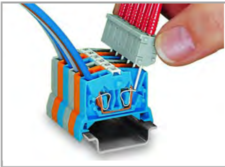
Testing by touch contact to the CAGE CLAMP® spring (limited to 0.5 A and 48 V test voltage) – test pins are not protected against accidental contact.
