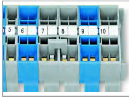
Commoning with comb-style jumper bar.
