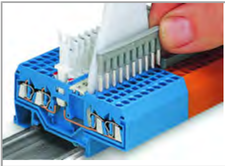
Commoning front-entry disconnect terminal blocks via comb-style jumper bar using a 10-pole operating tool.
