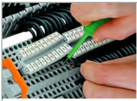
The flexible marker carrier, which is placed above the wiring level, can be pushed aside during wiring or commoning. The carrier has two staggered levels for WMB markers that perfectly align with the terminal block decks.
