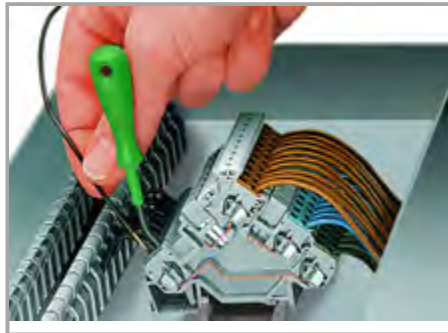
CAGE CLAMP® connection
