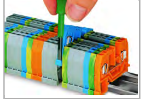
Removing a terminal block from the assembly.
