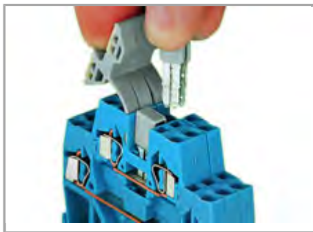
Commoning using an adjacent jumper (280-402).
