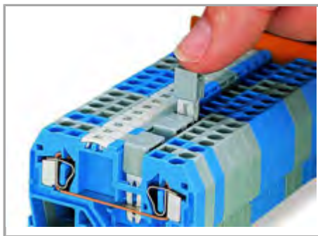
Commoning using an adjacent jumper (280-402) and alternate jumper (280-409). Push jumper down until fully inserted.
