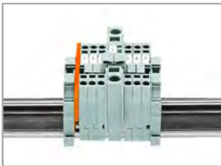
Commoning from 6 mm²/10 AWG (282 Series) to 1.5 mm²/16 AWG (279 Series) rail-mount terminal blocks via step-down jumpers.
