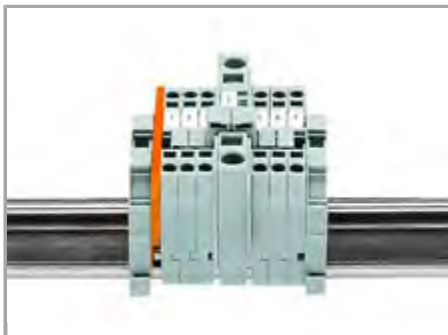
Commoning from 6 mm 2 /10 AWG (282 Series) to 1.5 mm 2 /16 AWG (279 Series) rail-mount terminal blocks via step-down jumpers.
