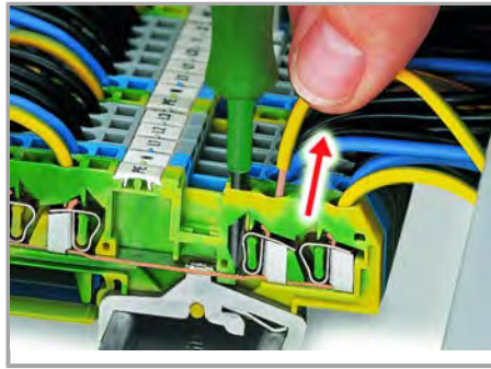
CAGE CLAMP® connection Removing a conductor.
