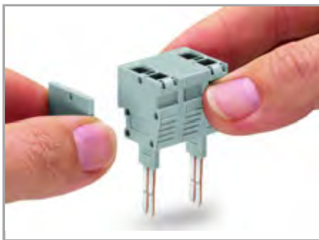
Snapping test plug and spacer modules (each with a spacer plate) together to assemble a multi-pole test plug module (max. 10 poles) for 10 mm terminal block width.
