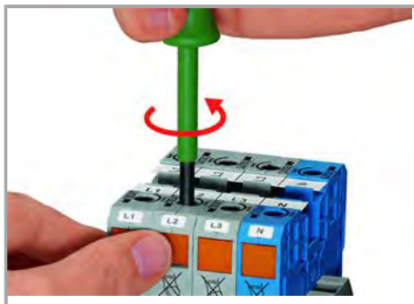
Conductor termination – step 1
