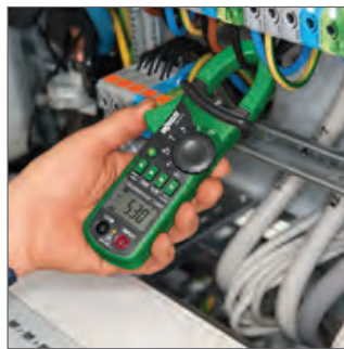
Clamp on meter for current measurement
