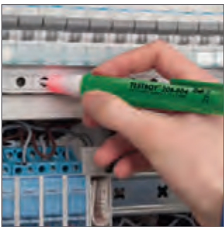
Testboy illuminates with voltage present
